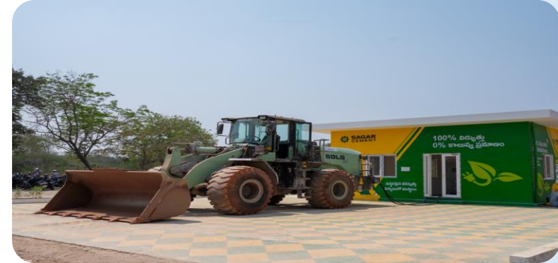
Electric Vehicles used for material handling at Dachepalli Plant, Andhra Pradesh
