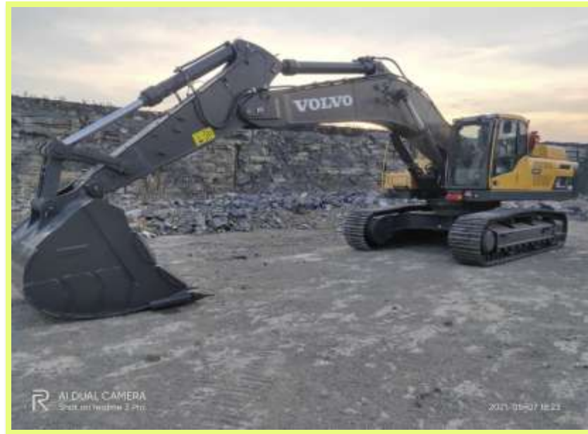
Volvo, Back hoe 2.8 Cu Mtr bucket shovel
