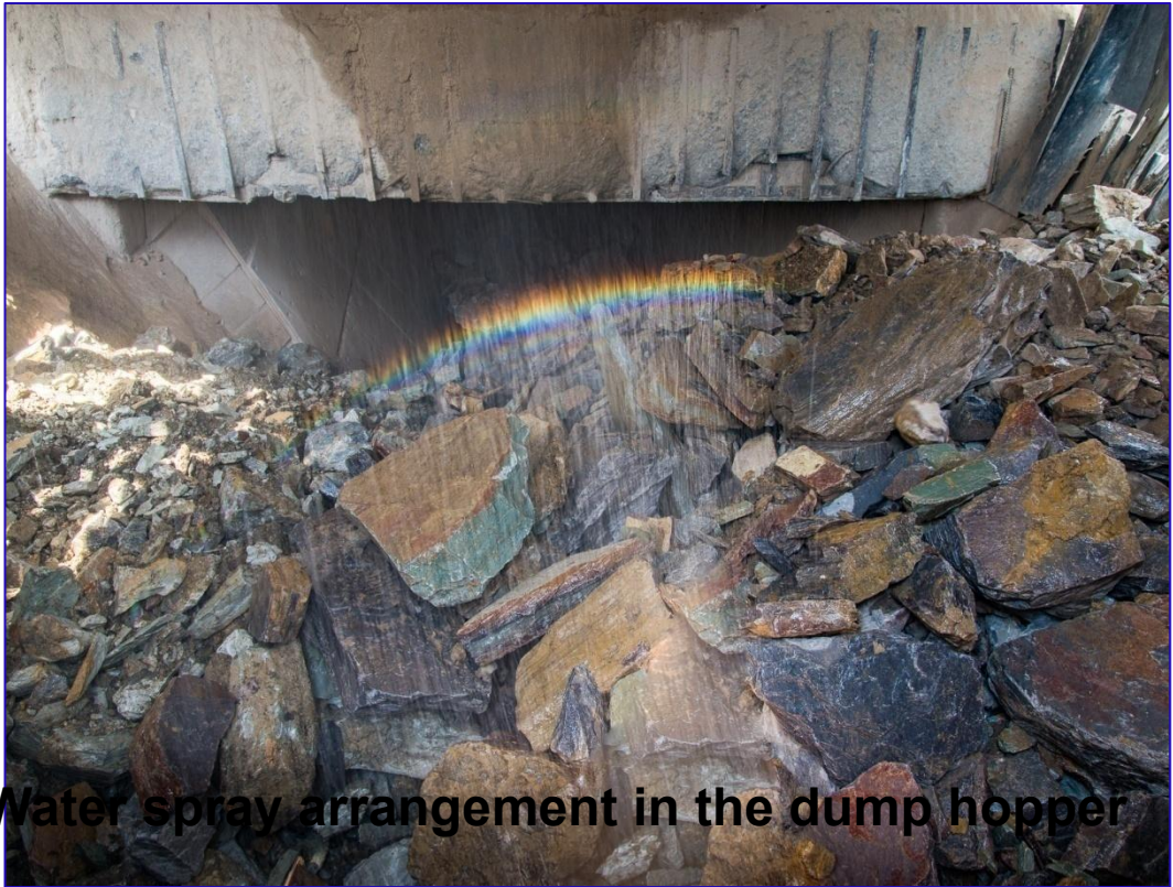
Water sprinkling in the dumper body material
