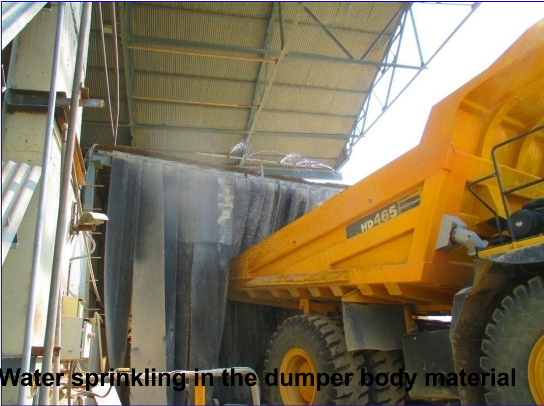
Water spray arrangement in the dump hopper
